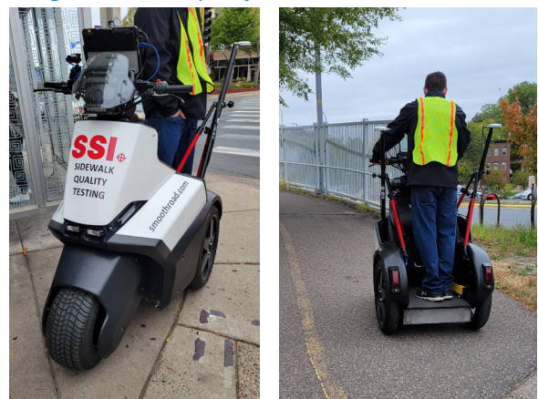
Figure A-4: Example of SEGWAY used to collect data
