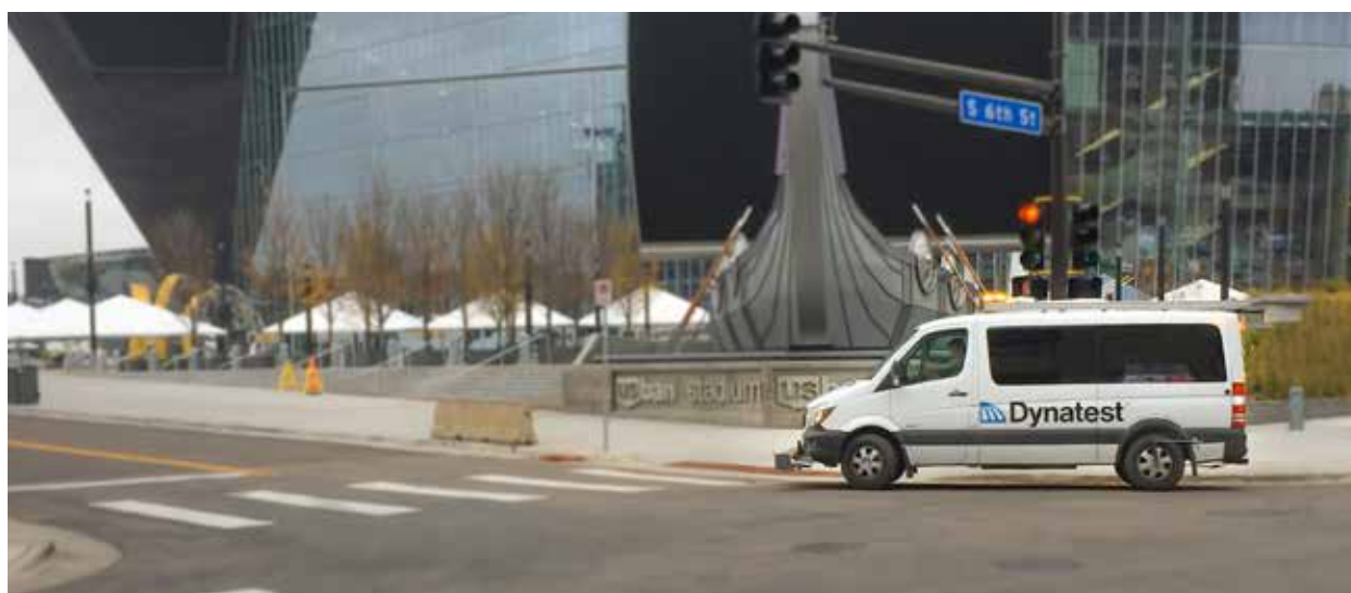
Figure 4 A Dynatest van collects pavement condition data in Minneapolis.
