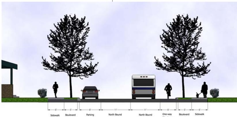
Scenario 1 shows a street design that requires minimal reconstruction of the street because the changes occur by and large within the existing street curbing. Existing lane widths, currently wider than necessary, would be narrowed to the city standard. This in and of itself would have the effect of slowing traffic. Narrowing traffic lanes creates sufficient space to allow the addition of the one-way on-street bike lane. Sidewalks would remain in their current locations. In
